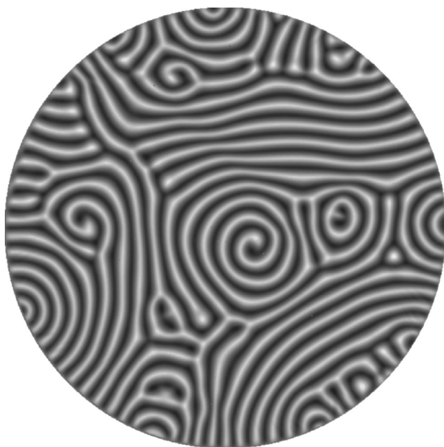
FIG. 1. Example of spiral defect chaos observed in a numerical simulation described in Sec. II C with insulating and no-slip boundaries, and with a spatial resolution of \Delta x=1/8 and a temporal resolution of \Delta t=10^{-3} . The mid-plane temperature field is plotted at time t=500 for parameters \epsilon=1.0 , \sigma=1 , and in a cylindrical geometry of aspect ratio \Gamma=30 . Dark regions correspond to cold sinking fluid, light regions to hot rising fluid. The spiral defect chaos planform is characterized by a disordered collection of spirals rotating in both directions and coexisting with dynamical defects such as grain boundaries and dislocations.
